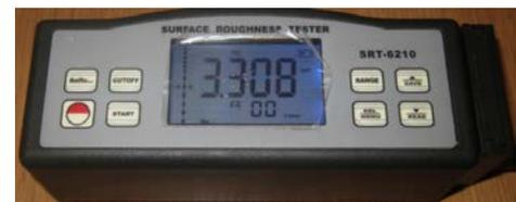
(c) Surface roughness tester (off-line measurement)
